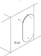
5. Complete all required electrical connections in the included electrical junction box and hang the mirror on screws.
