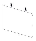
6. Place screws into the keyholes on the back of the mirror. Once all screws are positioned in keyholes, push mirror down to secure.
