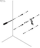
4. Insert screw anchors suited to the type of wall to which the mirror will be fixed. (Only screws in the case of wood studs).
