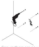
3. Ensure there are no water or electrical sources behind the fixing points and drill wall as per markings.
