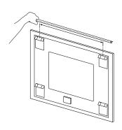
1. Measure the anchor positions taking consideration of the position of the mounting holes.
